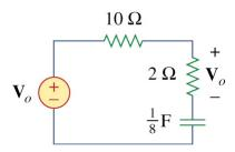
$\mathbf{H}(\omega) = \frac{\mathbf{V}_0}{\mathbf{V}_i}$ . This is a series RLC circuit, and therefore a voltage divider.
