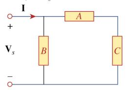
Element A:  $P_A = 2kW@power factor of 0.8 lagging.$
