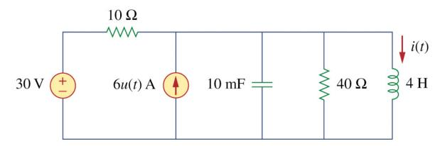
When the current source is off (for t < 0), the branch is an open circuit.
