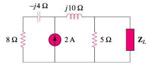
**2:** Repeat problem 4 by treating  $\mathbf{Z}_L$  as the load and using Thevenin's Theorem. You will find the Thevenin impedance and the (sinusoidal) Thevenin voltage. *Hint: Do not panic! Just do what you would do with resistors using the complex impedance of the elements.*
