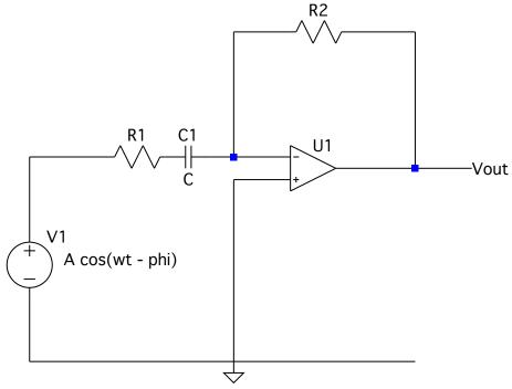
6.1 Express the input impedance  $\mathbf{Z}_i$  as a function of the angular frequency of the source,  $\boldsymbol{\omega}$ .
